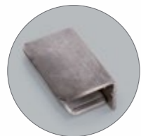
Rough pocket to be welded
